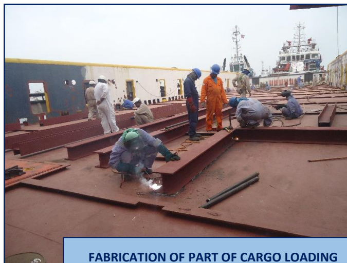
FABRICATION OF CARGO LOADING PLATFORM AT WORKSHOP
